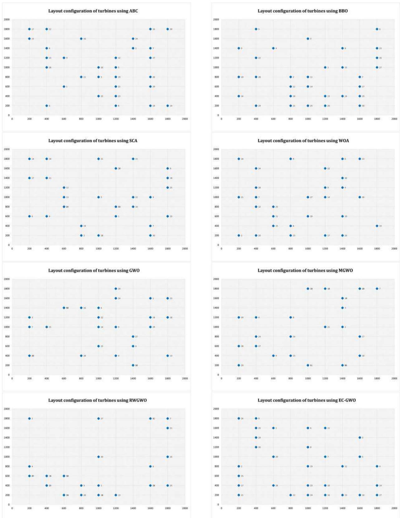
Fig. 9 Optimal configurations of 30 wind turbines
